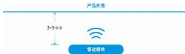
Figure 4 Distance between antenna surface and product housing
